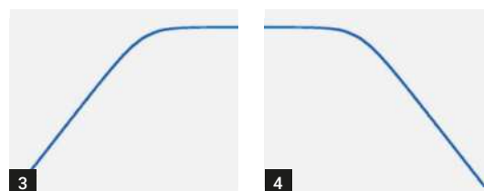
Fig. 1: Radio 4 long wave receiver project built on a 400-tie point protoboard. Fig. 2: Circuit diagram for the 198kHz long wave op-amp receiver. Fig. 3: Idealised frequency response of high pass filter (HPF). Fig. 4: Idealised frequency response of low pass filter (LPF). Fig. 5: NE5532 op-amp pinout (ON semiconductor datasheet). Fig. 6: NE5532 Open-loop frequency response taken from ON semiconductor datasheet. The discontinuity seen at 40dB is a drawing artefact, not an abrupt frequency shift. Fig. 7: NE5532 closed-loop frequency response taken from ON semiconductor datasheet with different value gain resistors (RF – feedback resistor).
