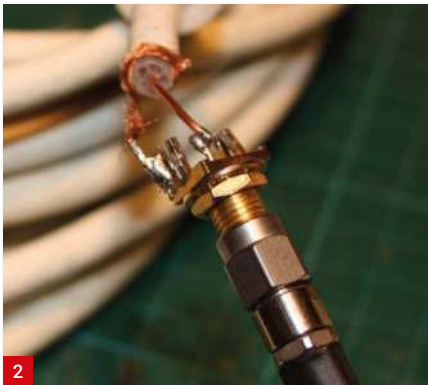
Fig. 1: NanoVNA displaying the TV coax measurement. Fig. 2: A TV coax cable with an SMA fitted. Fig. 3: An SDRKits VNWA plot comparing TV coax with a length of RG213. Fig. 4: The Termaline Dummy Load/Wattmeter. Fig. 5: A closer view of the Termaline front panel.
